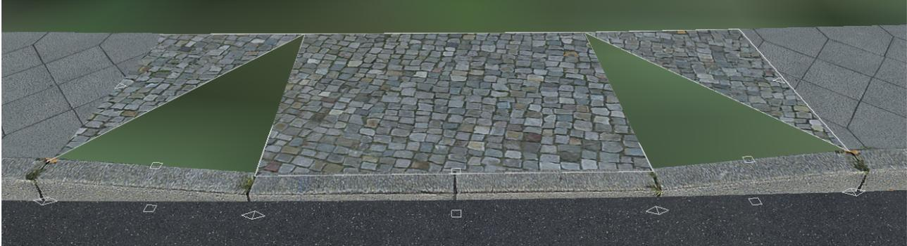
Because  $Z = -0.1$  was set for building this polygon the front points are at height  $-0.1$  and because of the vertical snapping the rear points are at  $0.0$ .
