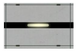
A currently active route leads over this route section. All route sections that are displayed in this way are "ready" for a trip to take place over them. At the same time, this means that no "hostile" route can be activated for this route section.
